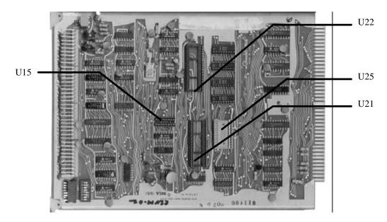
Take the Multigame Daughtercard and hold it so that the empty 40 pin socket is at the bottom, closest to you. Carefully place the Z-80 processor you removed from U22 into the socket on the Daughtercard. Pin one of the Z-80 should be in the lower-left corner and the "notch" of the IC should be on the left-side of the board like the EPROM above it on the Daughtercard. Press the Z-80 down firmly into the socket. Make sure you didn't miss any pins or bend any under.
